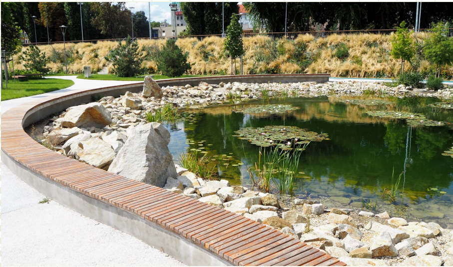
18 Elements of surface-level rainwater interception, e. g. lakes or basins, are suitable to be integrated with the overall spatial design framework and thus can naturally complement the visual identity of a public space while retaining its functional purpose. Bratislava, Park Jama
