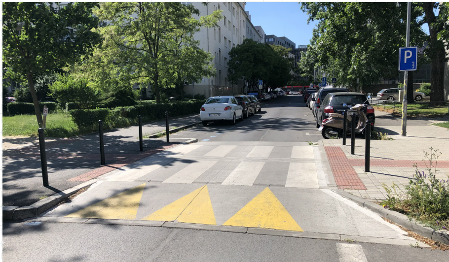
13 It is vital for pedestrian crossings in traffic-calmed and residential streets to be placed on the pavement level. Solutions like these increase safety and support movement without barriers. Bratislava, Bernolákova Street
