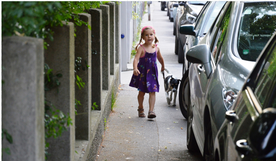
11 An unsuitable parking solution; a pavement which does not leave the minimum of 1,5m transitional width is non-permissible. Bratislava, Matičná Street
