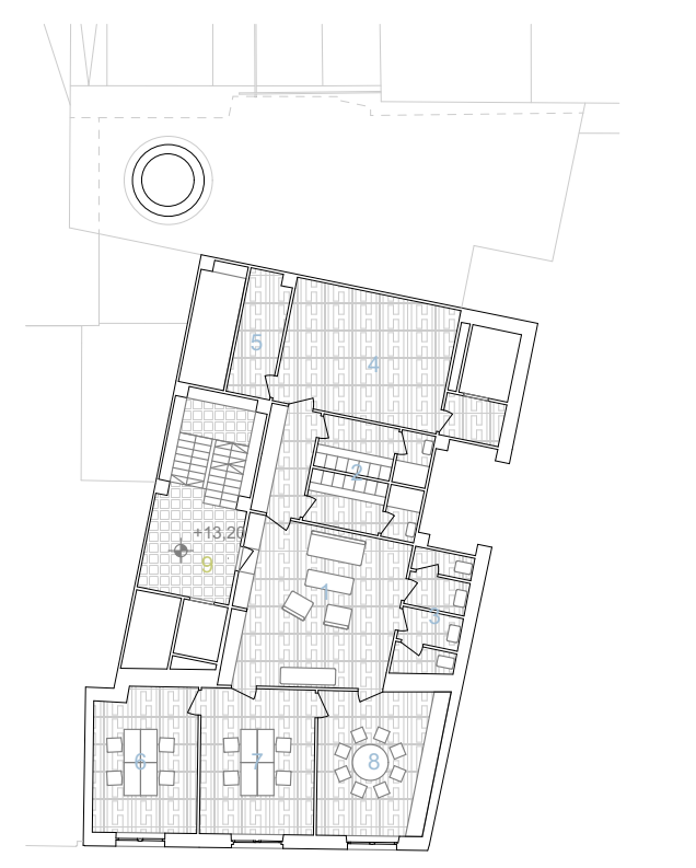
5TH FLOOR PLAN bath administration 1: chilling area 2: bath staff changing rooms 3: toilets 4: laundry and storage 5: cleaning storage 6: office 7: office 8: meeting room 9: public stairway
