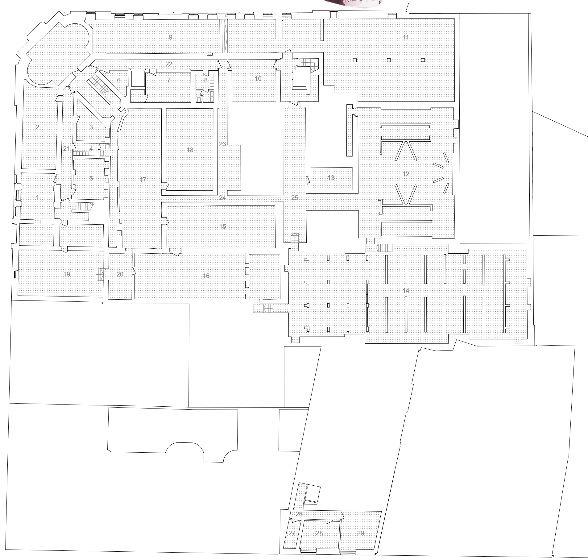
BASEMENT FLOOR PLAN 1: workshop 2: storage 3: garbage storage (bath) 4: maintenance staff social block 5: storage 6: garbage storage (bar) 7: storage and food preparation (bar) 8: bar staff social block 9-20: technical facilities 21-26: foyer 27-28: storage 29: garbage storage (bath)
